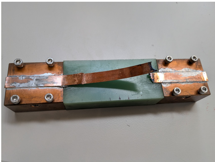
Figure 4.8: Photograph of the burnt HTS tape after exceeding critical current without quench protection.
