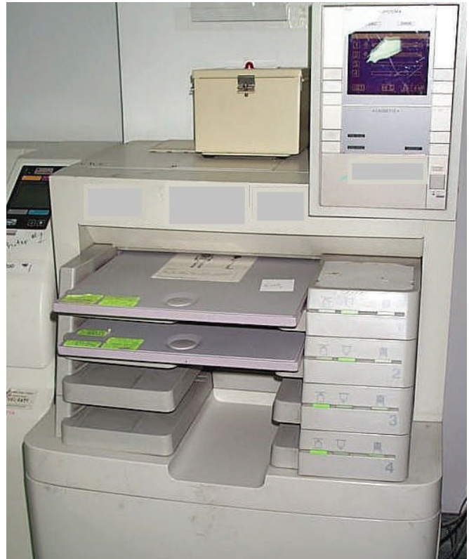
Figure 1b. The CR laser reader withdraws the fluorescent plate from the cassette and scans it.
