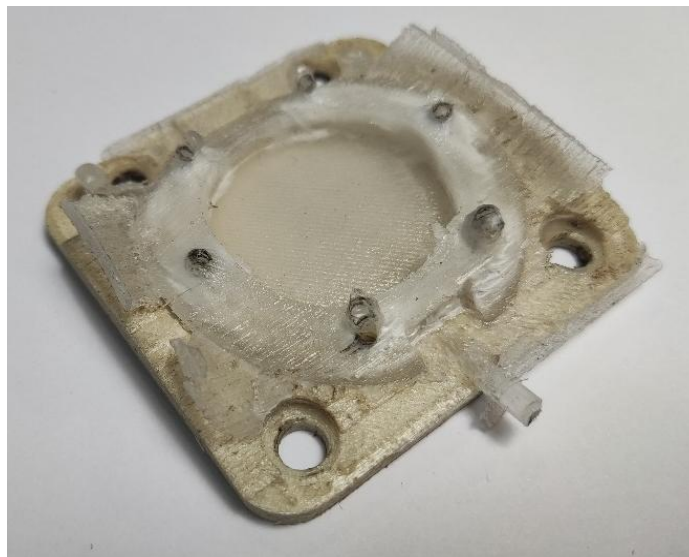
Figure 7.12 - Ejection side, case study 1, insert failure at first injection run.
