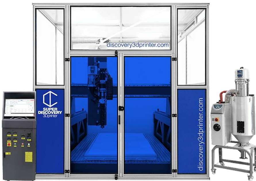
Figure 2.34 - Super Discovery 3D Granza, large scale FGF system [186].
