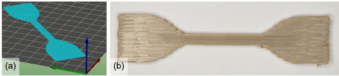
Figure 8.3 - Tensile test specimen (a) G-code simulation and (b) 3D printed.
