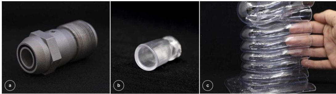
Figure 2.35 - (a): Hollow-Core 3D printing nozzle with a 24 mm orifice and a 2 mm wall thickness. (b): Extruded PETG bead. (c): 3D printed sample, cut, with a hand to represent scale and transparency, adapted from [193].
