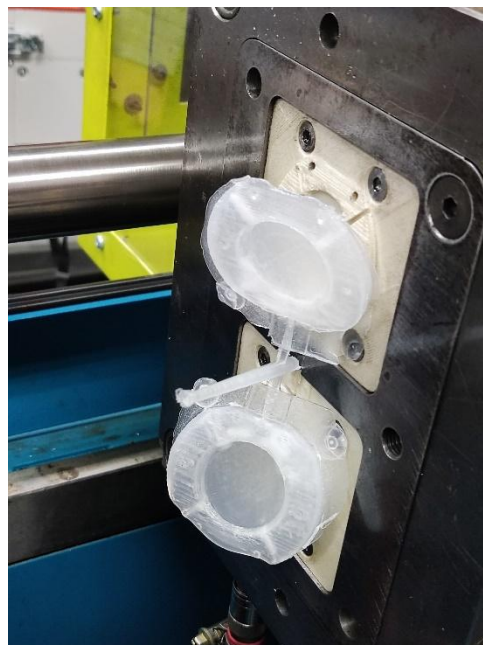
Figure 7.13 - Parts of case study 2 as produced during injection molding. The parts were stuck to the sides of the inserts due to flash, even after ejection
