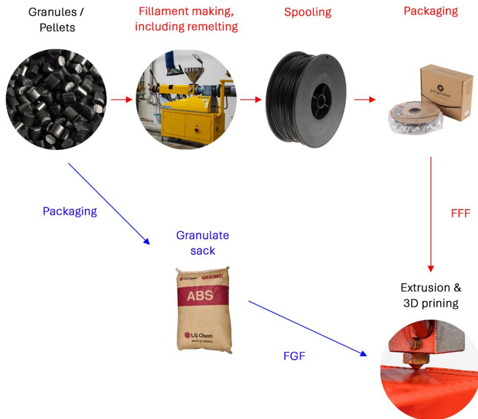
Figure 1.4 – Production process from raw material to 3D printing for FFF and FGF
