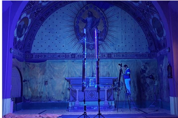
Figure 11. (left) During pre-production, the camera positions are determined and documented to achieve imaging consistency throughout the project. (right) Ultraviolet fluorescence image capture from predetermined Camera Position D. (Source: Own CAD design and photo)
