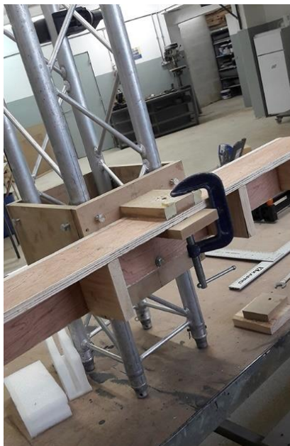
Figure 12. Projects pose different image acquisition challenges. Own design and build of custom vertical rig to capture three multi-nodal image mosaics from 36 predetermined camera positions (arranged as 4 columns with 9 rows). (Source: Own photos)
