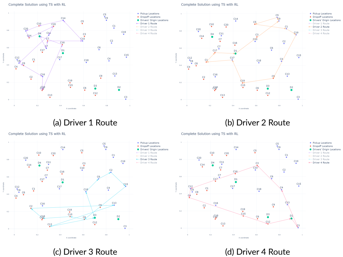
Figure 5.43 Drivers' Routes obtained using TS with RL on an instance with 4 drivers and 20 customers
