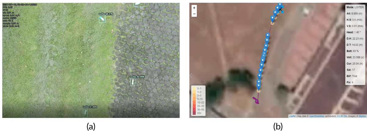
Figure 2.28 UAV trash monitoring results on the NTOU campus. (a) Detection results from the UAV. (b) Detected litter plotted on a map, showing real-time monitoring and detection. (Source: [124])
