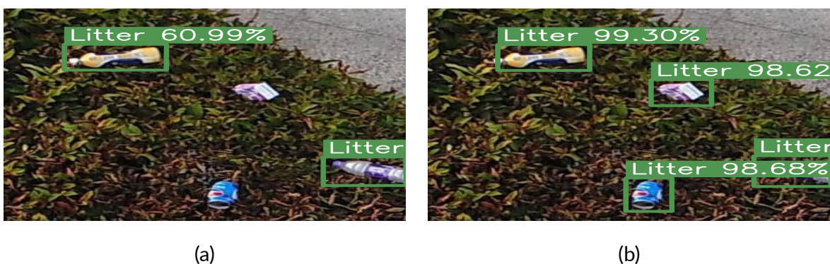
Figure 4.20 Sample predictions on test subset images from the FCOS detection model, trained on the SODA dataset and evaluated on the BDW dataset. Subfigure (a) shows outputs from the baseline model, while (b) presents predictions from the corresponding student model.
