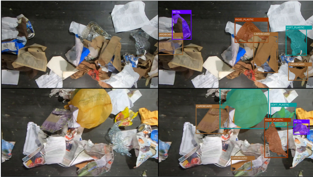
Figure 2.25 Sample images (left) and ground truth polygon annotations (right) in the ZeroWaste dataset. (Source: [8])
