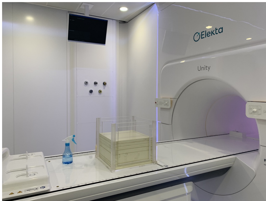
Figure 3.4: Film exposure set up which includes a total thickness of cm of solid water with the film inserted beneath the first 5 cm solid water blocks.
