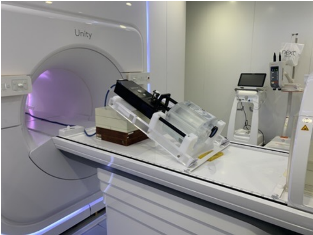
Figure 3.1: Modus QUASAR™ MRI 4D Phantom on MRL
