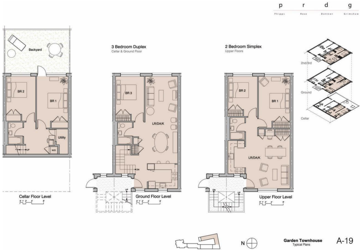
Figure 9 - Internal squarish layouts - enhance cross ventilation
