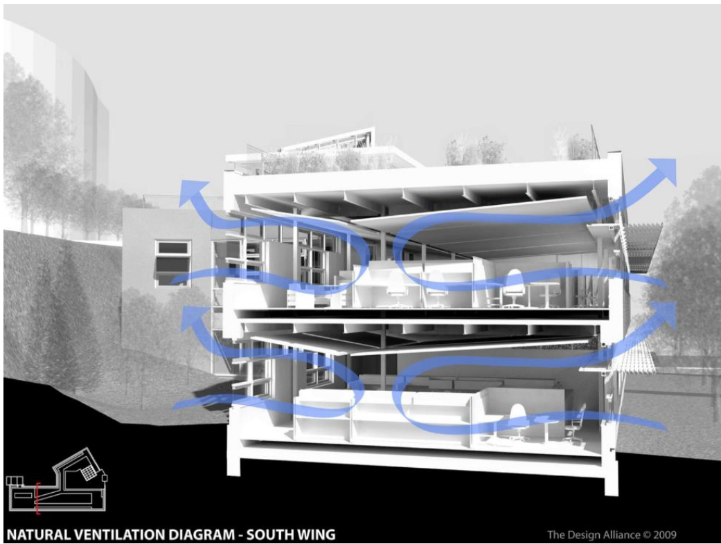
Figure 14 - Natural cross ventilation
