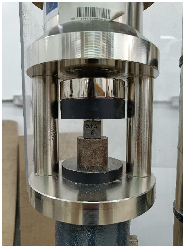
Figure 4.19 – Compression Machine used to measure Compressive Strength
