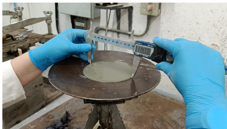
Figure 4.13 – Flow Table with Paste Mix & Vernier Calliper
