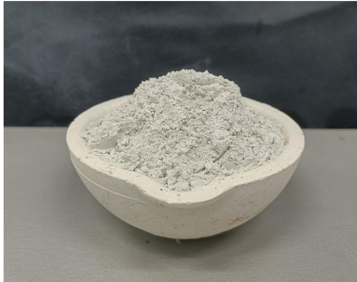
Figure 4.7 – Cl + Co W Ca 600 powder heated in a crucible
