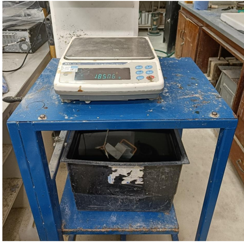
Figure 4.17 – Obtaining the Buoyant Mass of the Samples
