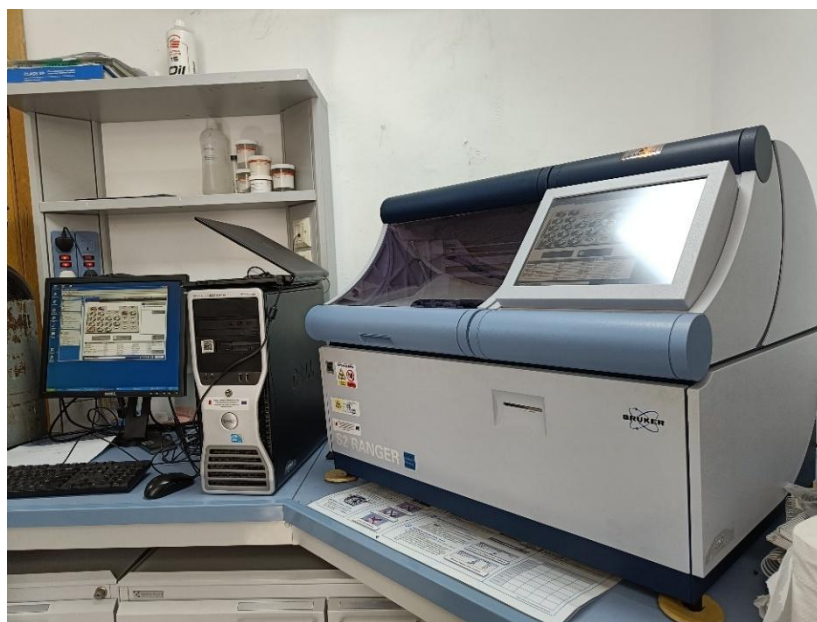
Figure 4.9 - Bruker ED-XRF X-Ray Fluorescence Spectrometer S2 Ranger
