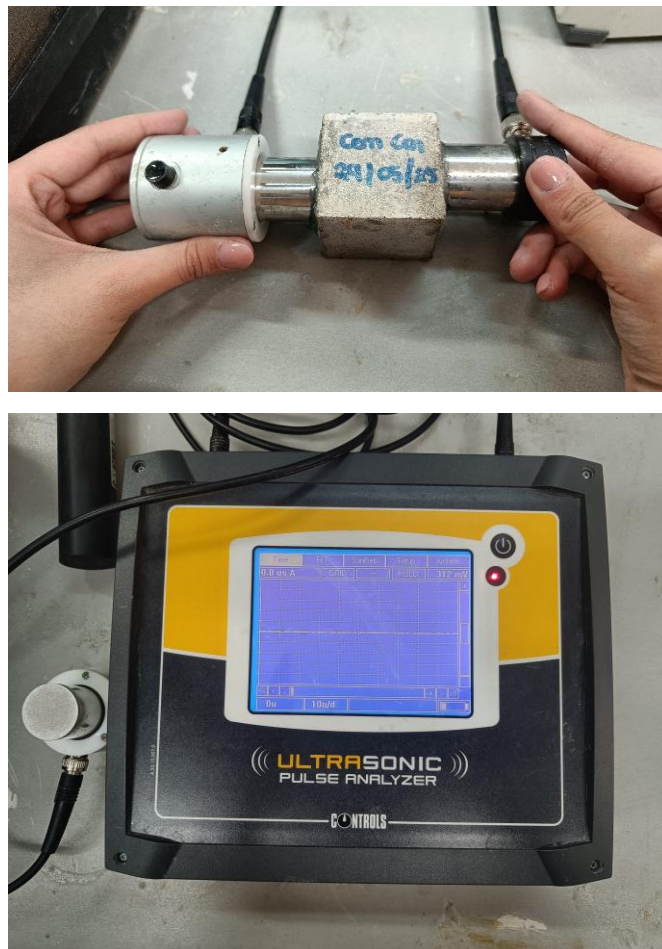
Figure 4.21 – Apparatus used in UPV Test
