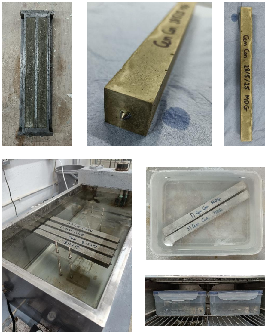
Figure 4.22 – Process of Accelerated Mortar Bar Test
