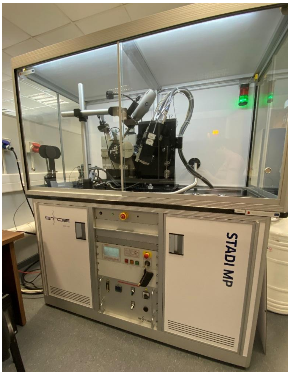
Figure 4.12 - STOE Stadi MP diffractometer equipped with a curved germanium (111) monochromator and a Mythen 1K detector
