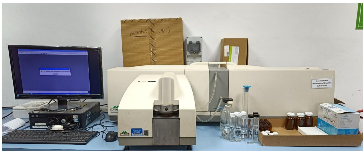
Figure 4.10 - Malvern Instruments Particle Size Analyser
