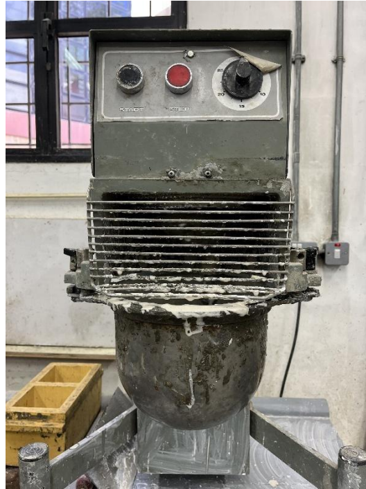
Figure 3.33 - The plaster mix was placed in the mixer so that any clumps of unmixed plaster were removed
