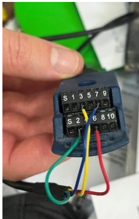
Figure 3.5 - A photo of the LVDT sensor connected to the RJ50 input, which was directly connected to the data logger
