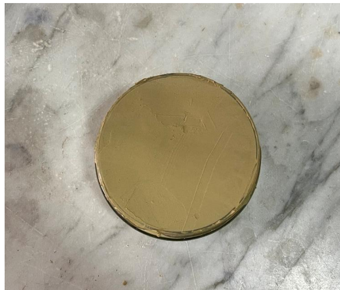
Figure 4.1 - A photo of the smooth clay surface inside the container
