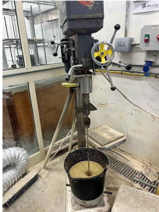
Figure 3.40 - A photo of the clay being mixed into a slurry using a pillar drill for 24 hours
