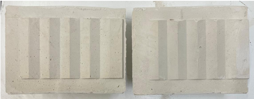
Figure 8.15- Bottom and top specimens for Test 8 before experimentation
