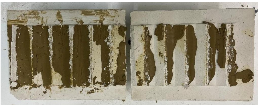
Figure 8.6- Bottom and top specimens for Test 3 after experimentation
