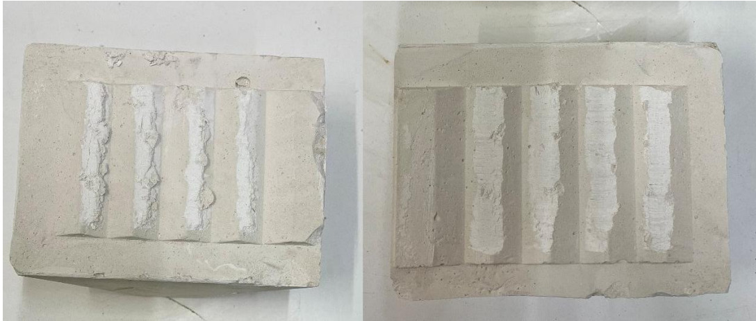
Figure 4.25 - The test results showing how the asperities have been sheared off
