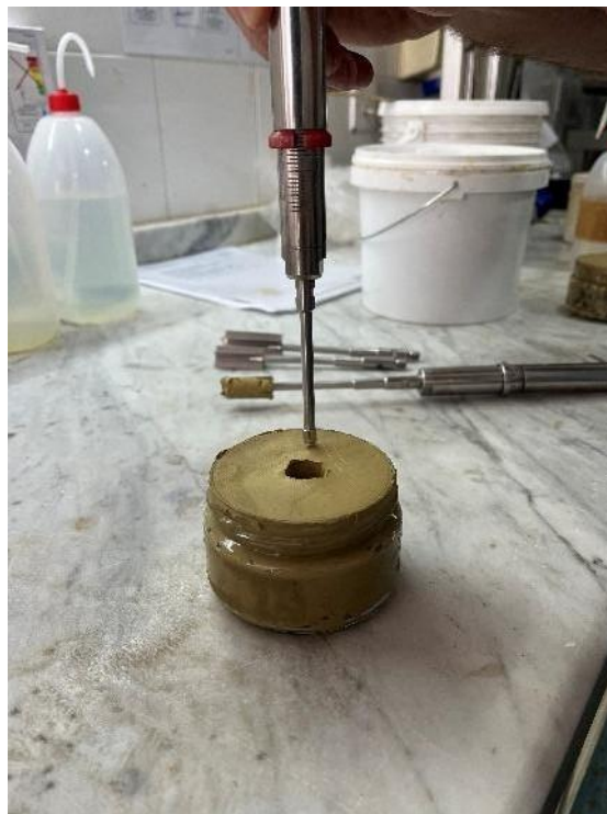
Figure 4.3 - A photo of the pocket penetrometer test as it was being inserted inside the container
