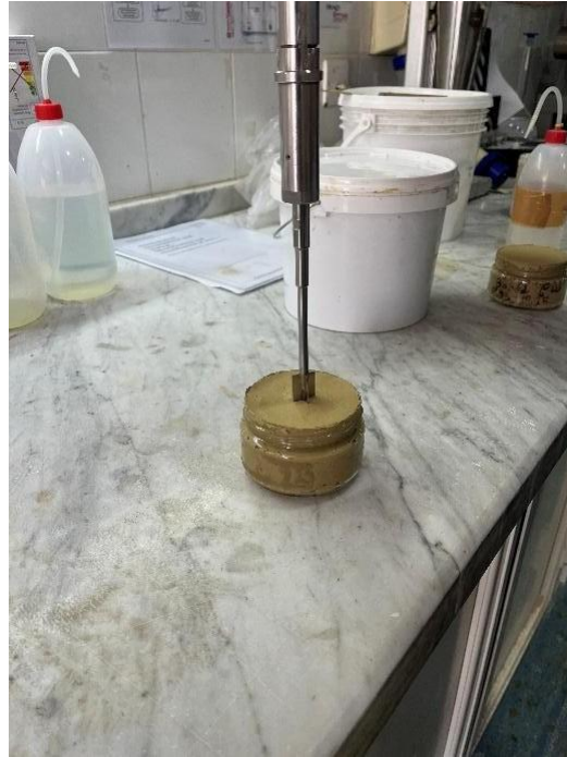
Figure 4.2 - A photo of the shear vane test as it was being inserted inside the container
