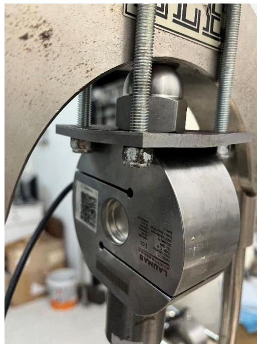
Figure 6.3 - The plate connecting the load cell to the arm visibly bent after testing
