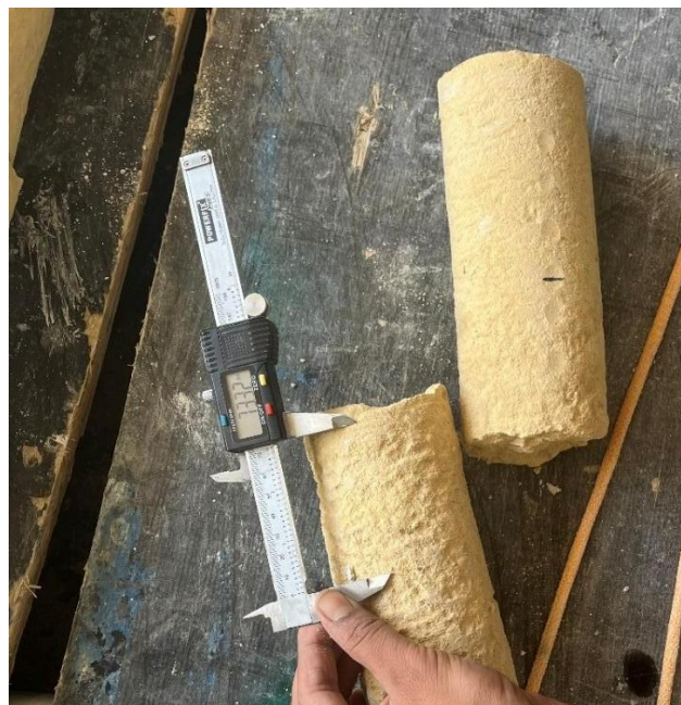
Figure 3.23 - A photo adjusting the actual size of the rock to fit the mould. The discontinuity is not cut out.
