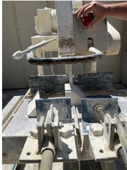
Figure 3.28 - The plaster volumes being extracted from the already tested specimen
