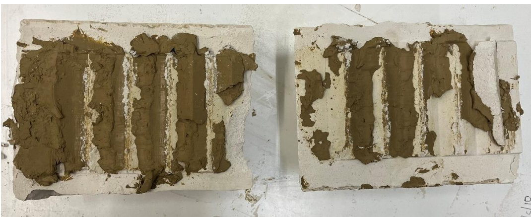
Figure 8.18- Bottom and top specimens for Test 9 after experimentation
