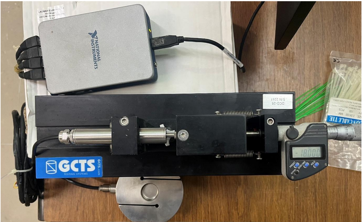
Figure 3.8 - The LVDT was attached to the micrometre where readings start being recorded. At this current instance the measured displacement from the micrometre was of 18mm.
