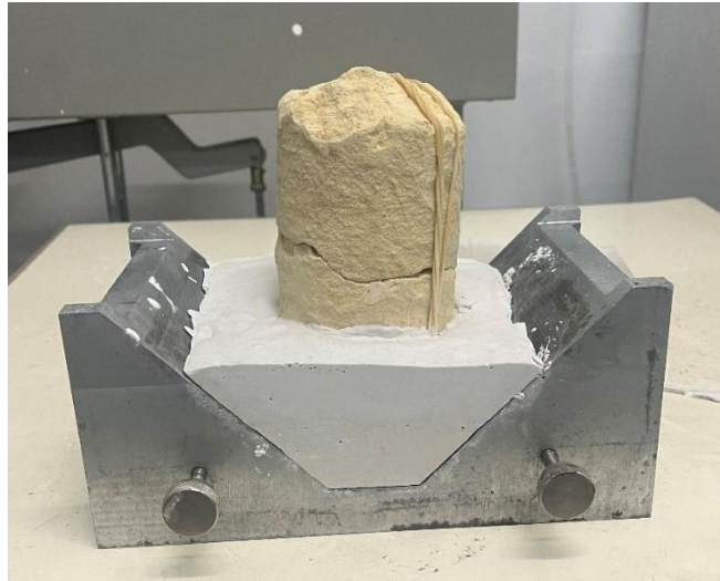
Figure 3.24 - A photo showing the rubber bands used to keep the rocks in place as the mould is being cast. This plaster solution holding the rock specimen is then encased in the Direct Shear Box as shown in Figure 3.1.
