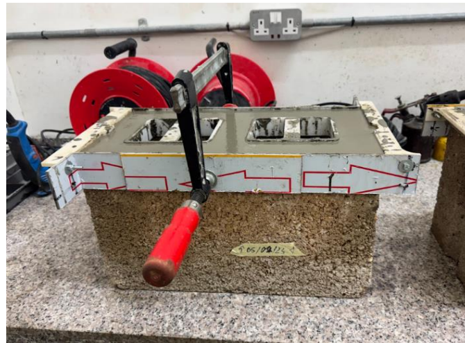
Figure 3.7: Capping Moulds and Set-Up
