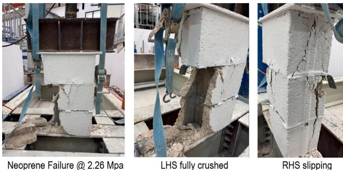
Figure 4.26: Images of Neoprene Full Wallette Failure
