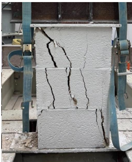
M6 (double cap) Failure
