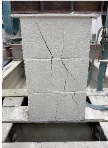
M6 Failure @ 2.32 Mpa
