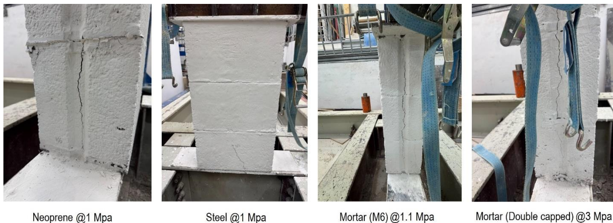
Figure 4.18: Images of Initial Cracking of Shell Bedded Wallettes.
