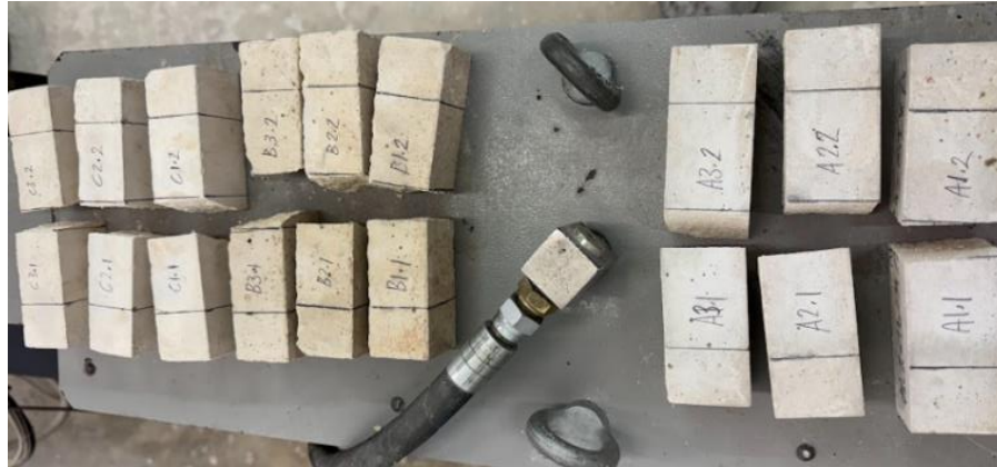
Figure 3.4 : Mortar compressive test samples obtained after flexural tests
