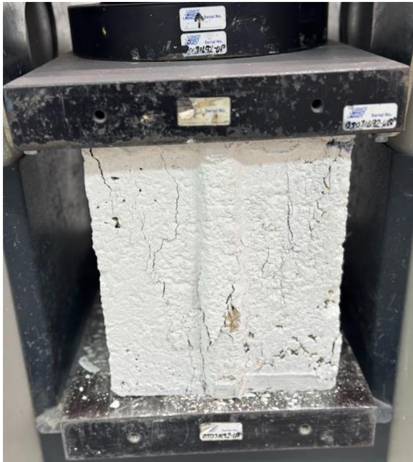
Figure 4.1: Specimen G Crushed Block in Compressive Rig, Failure @5.34 MPa
