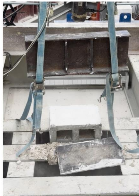
M6 Mortar (double cap) @5.3Mpa
