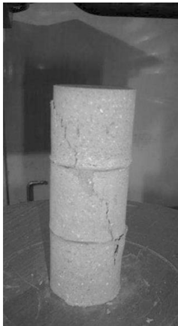
Figure 2.11: Vertical Cracks in Core sample (Drougkas et al, 2015)
