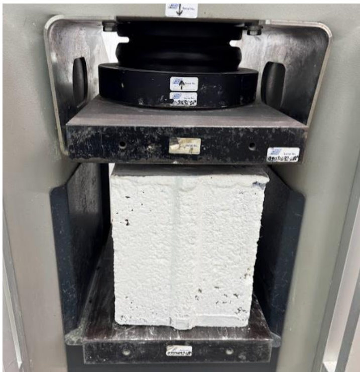
Figure 3.9 : Compressive Test Set Up of Hollow Concrete Blockwork.
