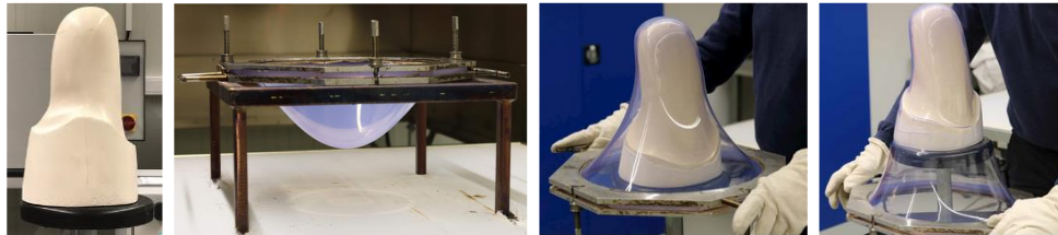
Figure 3.6: Images show part of the process required in making a patient's socket
