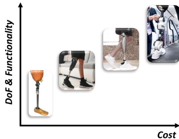
Figure 3.4: Graph shows examples of prosthesis on a plot of DoF and functionality against cost
