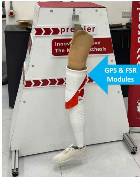
Figure 8.20: Location of GPS module and FSR
