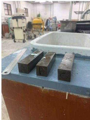
Figures 4.37 and 4.38: Measuring, weighing, and marking of three prism samples
