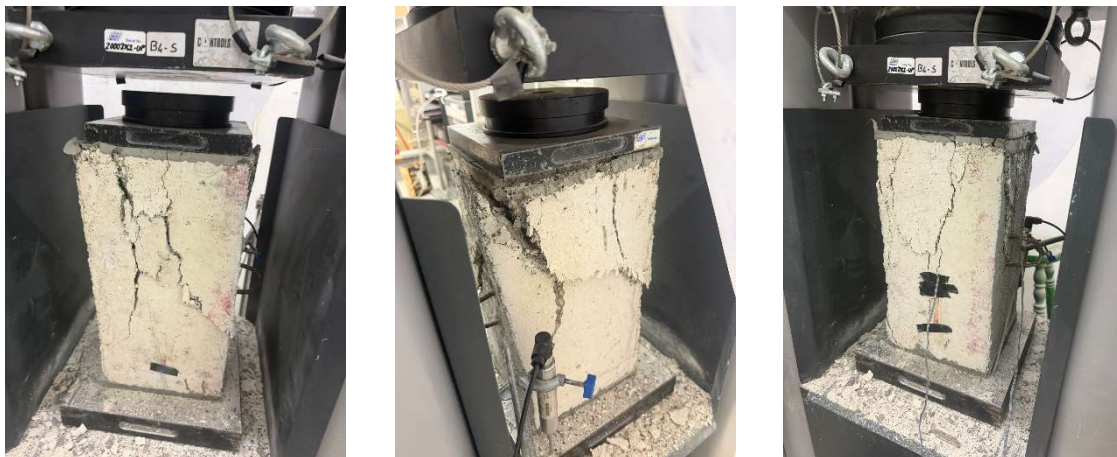
Figure 5.28: CR25 short column failure
