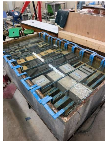
Figures 4.23 and 4.24: Cubes after de-moulding / Curing process of cubes
