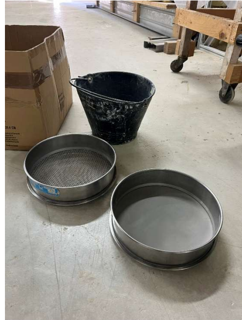
Figures 4.3 and 4.4: Sieves present at Faculty laboratory / 4mm and 63 \mu m sieves used to sieve crumb rubber
