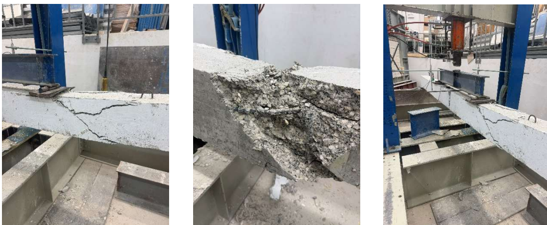
Figure 5.17: CR25 beam failure
