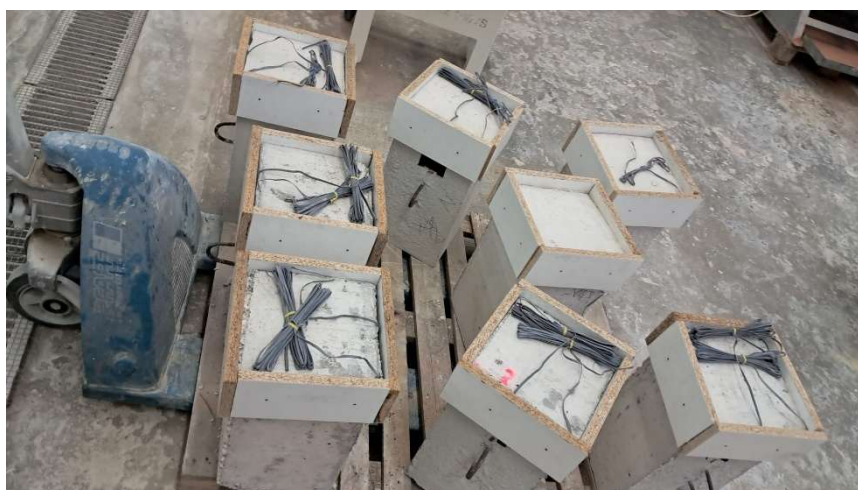
Figure 4.25: Capping layer moulds attached to short column ends
