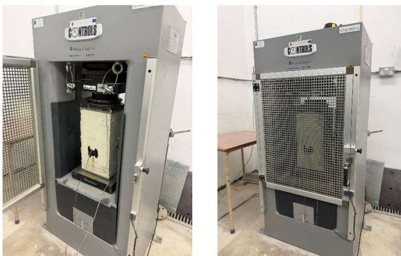
Figure 4.36: Short column compressive strength testing set-up
