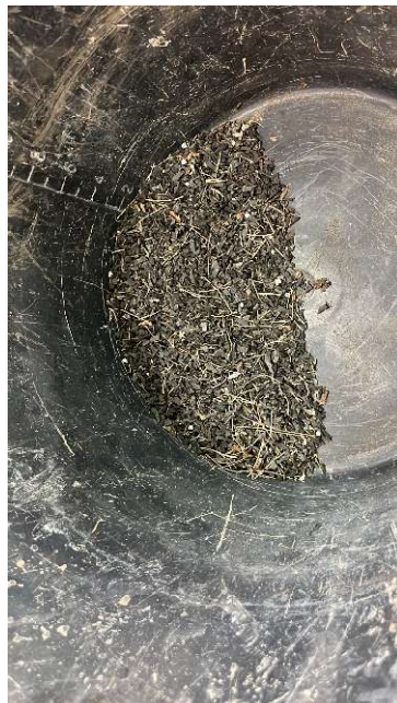
Figure 4.5: Excess foreign materials and silts filtered out through sieving crumb rubber
