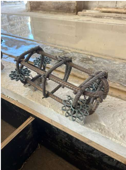
Figures 4.11, 4.12, and 4.13: Short column reinforcement cage / Attachment of steel strain gauge / Addition of melted wax layer to strain gauge
