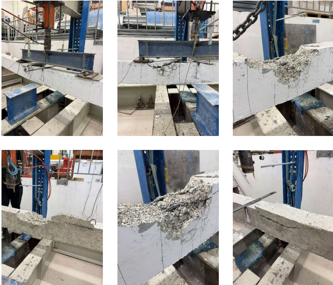
Figure 5.11: CR25 beam failure
