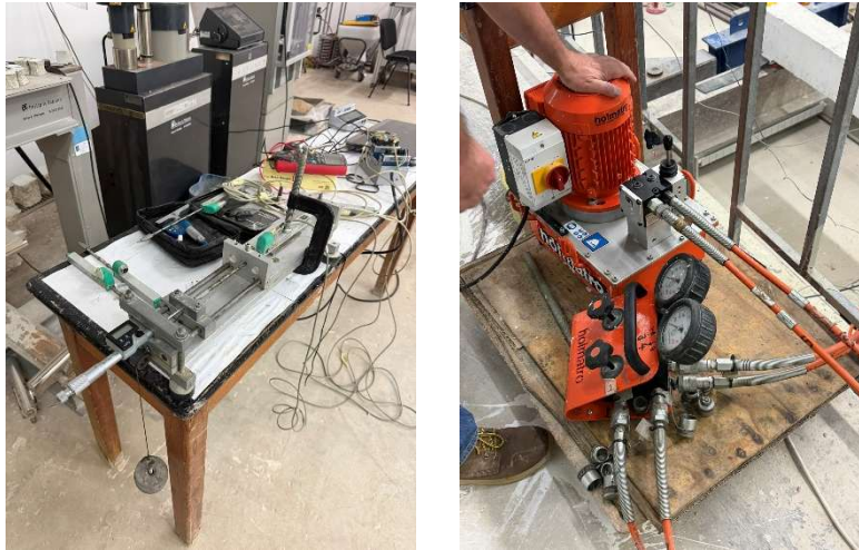
Figures 4.31 and 4.32: Preparation of LVDTs / Hydraulic jack
