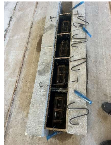
Figures 4.14, 4.15, and 4.16: Pre-oiled plastic cube moulds / Beam moulds with steel cages / Short column moulds with steel cages
