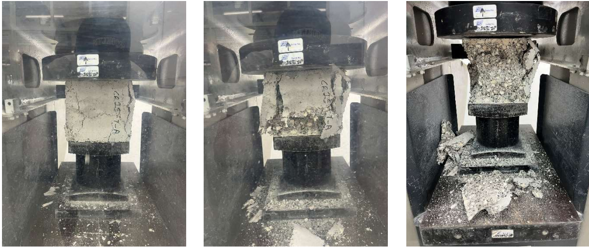
Figure 5.2: Crushed cubes – CR25 design mix
