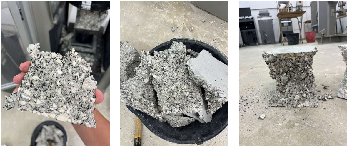
Figure 5.3: Evidence of weak mechanical bonding (ease of crumbling) – CR25
