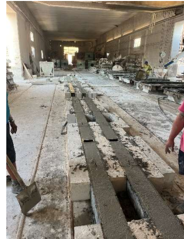
Figures 4.17, 4.18, and 4.19: Casting process / Vibrating of concrete / Addition of hooks for ease of transportation
