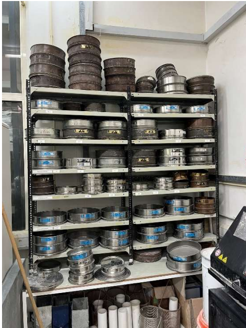
Figures 4.3 and 4.4: Sieves present at Faculty laboratory / 4mm and 63 \mu m sieves used to sieve crumb rubber
