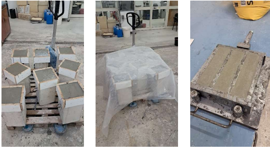
Figures 4.26, 4.27, and 4.28: Sika S55 capping layer cast / Polythene sheeting cover to prevent water evaporation / Casting of prism samples in steel moulds
