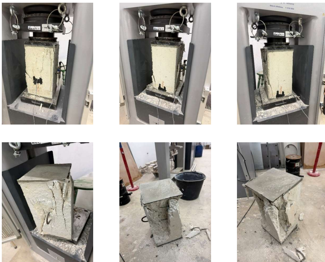
Figure 5.23: CM short column failure
