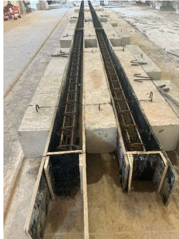
Figures 4.14, 4.15, and 4.16: Pre-oiled plastic cube moulds / Beam moulds with steel cages / Short column moulds with steel cages
