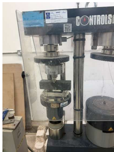
Figure 4.39: Three-point flexural test set-up
