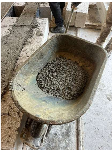
Figures 4.20, 4.21, and 4.22: Mix sample used for cube casting / Compacting concrete cubes with a tamping rod / Labelling of samples
