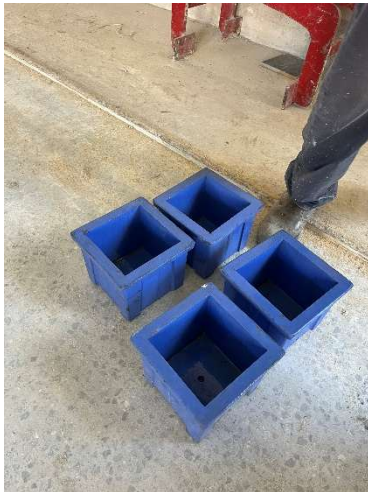
Figures 4.14, 4.15, and 4.16: Pre-oiled plastic cube moulds / Beam moulds with steel cages / Short column moulds with steel cages
