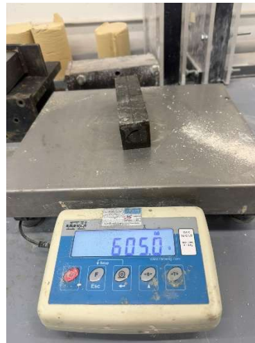
Figures 4.37 and 4.38: Measuring, weighing, and marking of three prism samples
