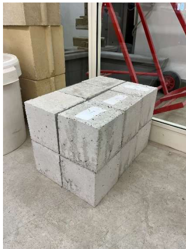
Figures 4.23 and 4.24: Cubes after de-moulding / Curing process of cubes
