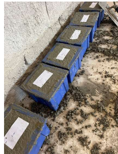
Figures 4.20, 4.21, and 4.22: Mix sample used for cube casting / Compacting concrete cubes with a tamping rod / Labelling of samples
