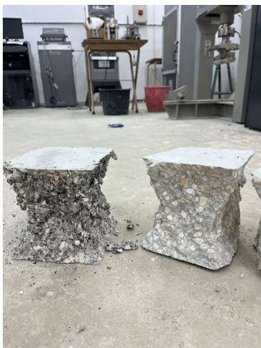
Figures 5.4 and 5.5: Crushed CR25 vs CM / Failure of CM vs CR25
