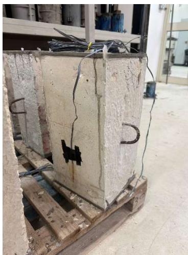
Figure 4.35: Position of concrete strain gauge on short column sample
