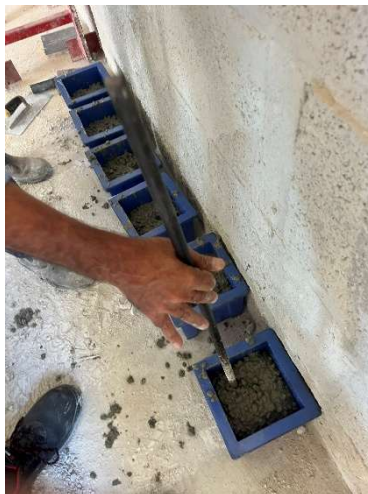
Figures 4.20, 4.21, and 4.22: Mix sample used for cube casting / Compacting concrete cubes with a tamping rod / Labelling of samples
