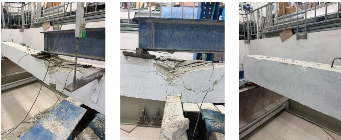
Figure 5.16: CM beam failure
