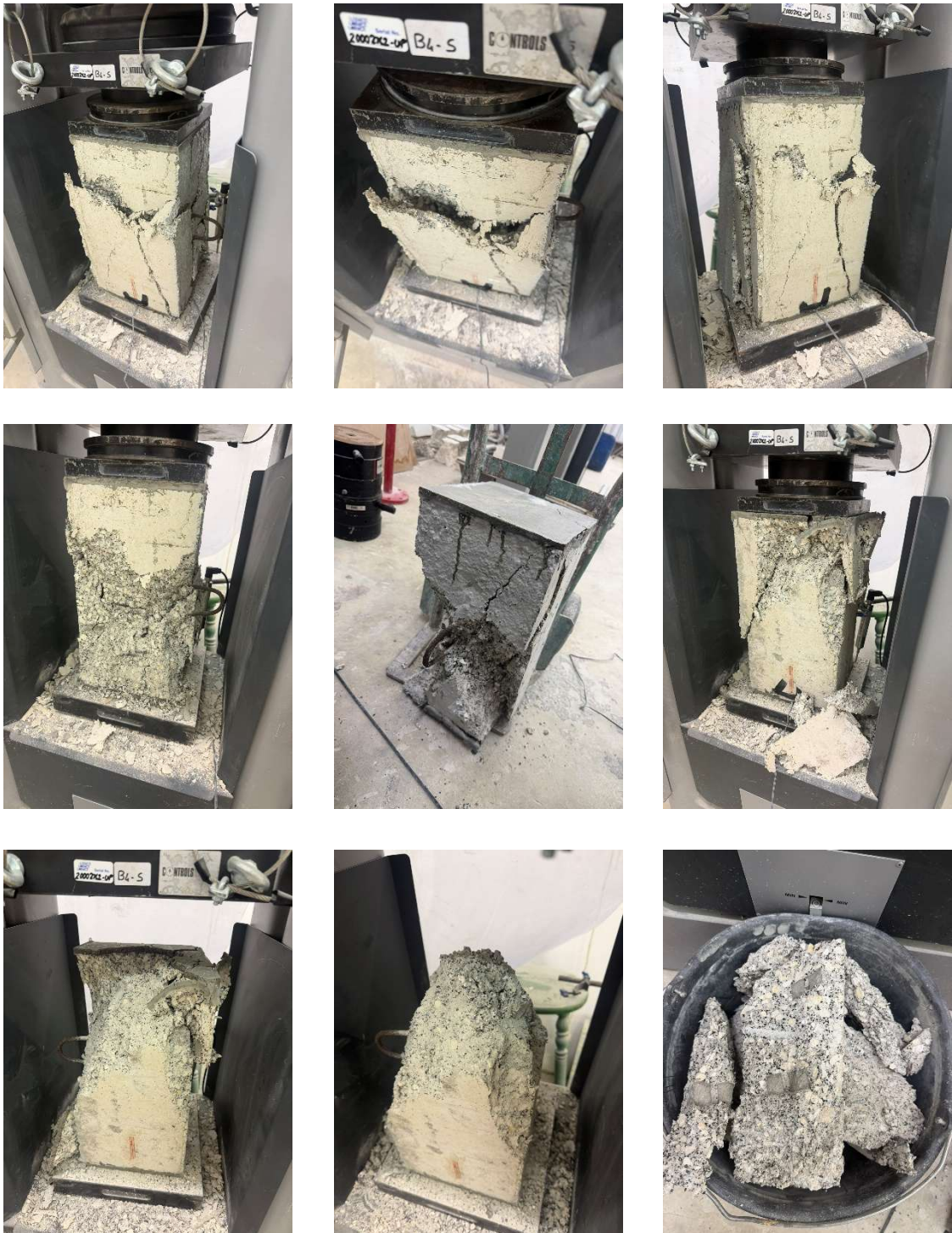
Figure 5.24: CR25 short column failure
