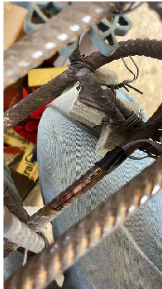
Figures 4.11, 4.12, and 4.13: Short column reinforcement cage / Attachment of steel strain gauge / Addition of melted wax layer to strain gauge
