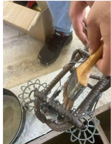
Figures 4.11, 4.12, and 4.13: Short column reinforcement cage / Attachment of steel strain gauge / Addition of melted wax layer to strain gauge
