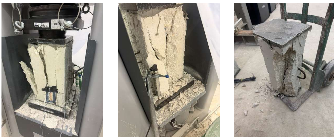
Figure 5.27: CM short column failure
