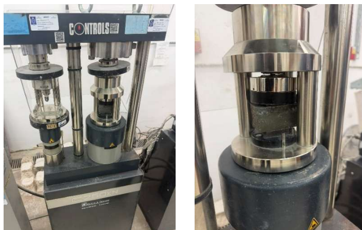
Figure 4.40: Compressive strength test set-up
