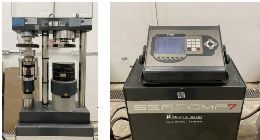
Figure 31 - Compression Machine Set Up
