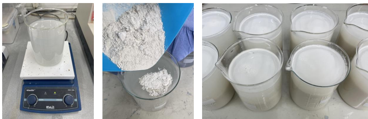
Figure 12 – Slaked Lime being Dissolved (Left), Raw Material Poured into Solution (Middle) and Raw Material within the Limewater Solution
