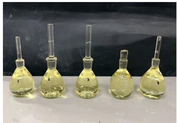
Figure 18 – Pycnometers filled with De-aerated Distilled Water (Left) and Pycnometers filled with Redistilled Kerosine (Right)
