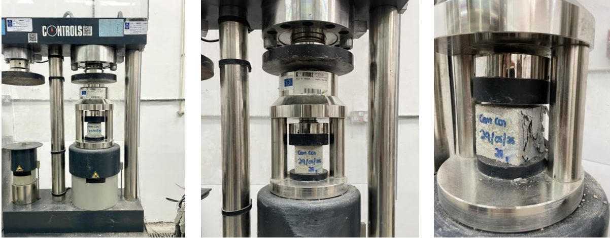
Figure 40 - Compression Machine Set Up (Left), Sample Loaded in Compression Machine (Middle) and Crushed Sample (Right)
