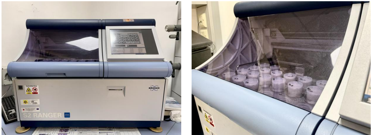
Figure 22 - Bruker S2 Ranger Device (Left) and Tested Samples within Apparatus (Right)
