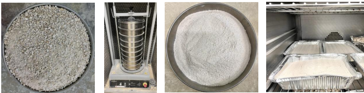
Figure 2 – Material after Los Angeles (First), Sieve Shaker (Second), Sieved Material (Third), Oven Drying Material (Fourth)
