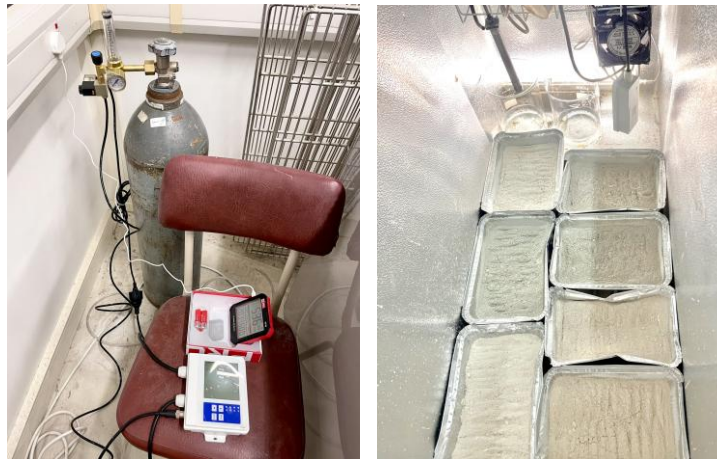
Figure 7 - Dry Carbonation Set Up Outside Chamber (Left) and Inside Chamber (Right)
