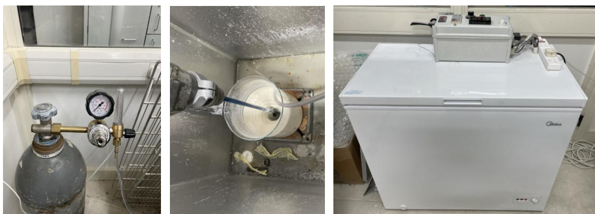
Figure 10 - Flow Meter (Left), Dry Carbonation Set Up Inside Chamber (Middle) and Chamber (Right)
