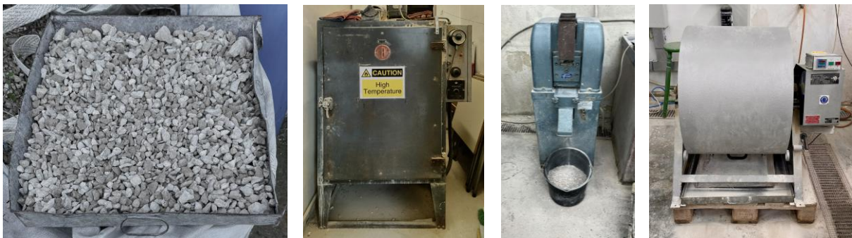
Figure 1 - Recycled Concrete Material (First), Oven (Second), Jaw Crusher (Third), Los Angeles Machine (Fourth)
