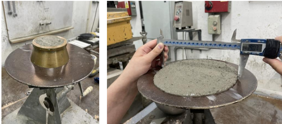
Figure 36 - Mortar Mix Poured into Conical Mould (Left) and Measured Diameter of Spread after Tamping (Right)
