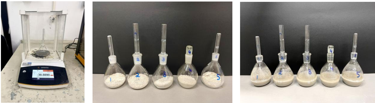
Figure 19 – Pycnometer and Stopper weighed Empty (Left), Cement Placed within Pycnometer (Middle) and Redistilled Kerosine Poured within Pycnometer (Right)
