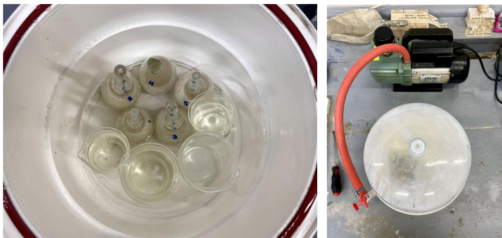
Figure 20 – Pycnometers and Beakers within Desiccator (Left) and Vacuum Desiccator Set Up (Right)
