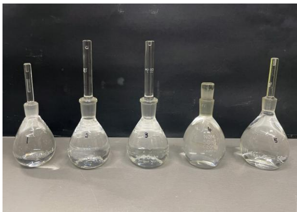
Figure 18 – Pycnometers filled with De-aerated Distilled Water (Left) and Pycnometers filled with Redistilled Kerosine (Right)
