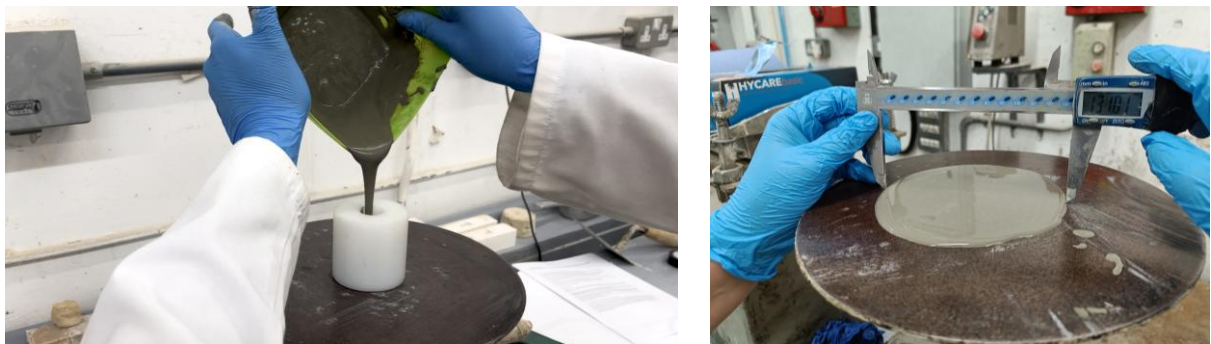
Figure 28 - Paste Mix Poured into Conical Mould (Left) and Measured Diameter of Spread after Tamping (Right)
