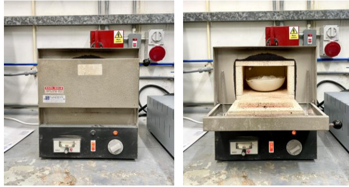
Figure 6 - Muffle Furnace (Left) and Material to be Calcined (Right)
