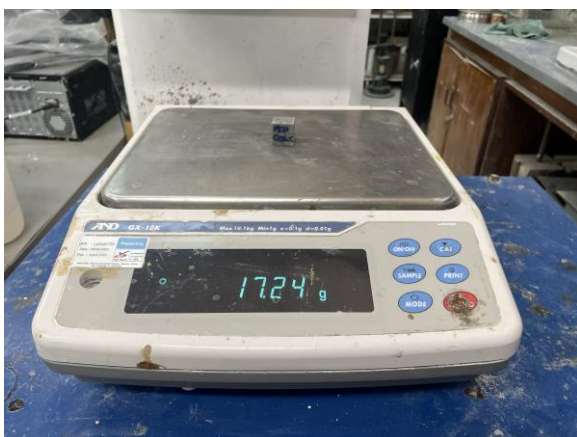
Figure 33 - Saturated Surface-dry Mass of Sample (Left) and Buoyant Mass of Sample (Right)
