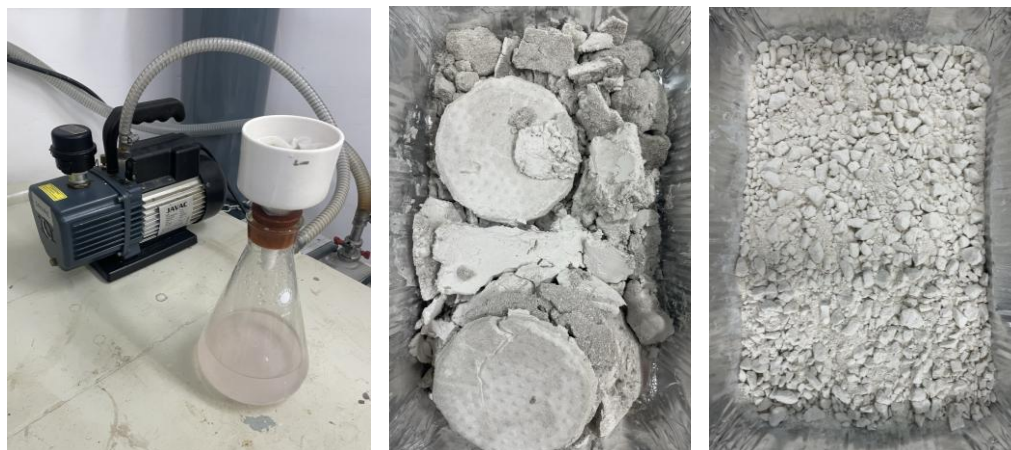
Figure 11 - Vacuum Pump Filtration (Left), Retained Material (Middle) and Dried/Crushed Material (Right)
