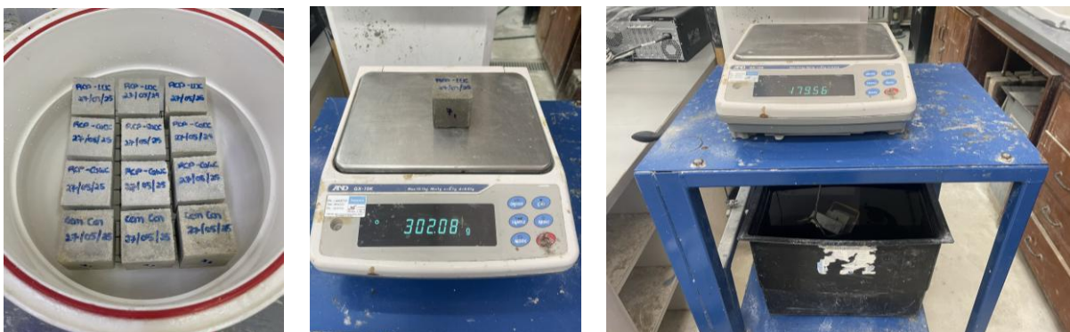
Figure 37 – Samples Placed within Test Set Up (Left), Saturated Surface-dry Mass of Sample (Middle) and Buoyant Mass of Sample (Right)
