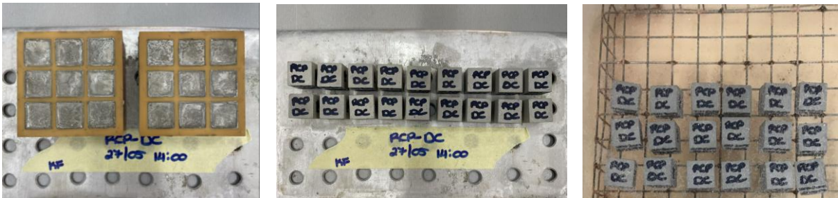
Figure 15 – Curing of Cubes at Ambient Temperature (Left), Demoulding of Cubes (Middle) and Curing within Water Bath (Right)
