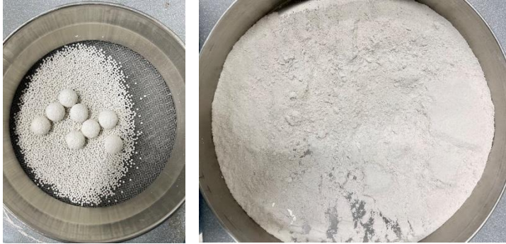
Figure 4 – Steel Balls and Beads (Left) and Raw Powder Material (Right)
