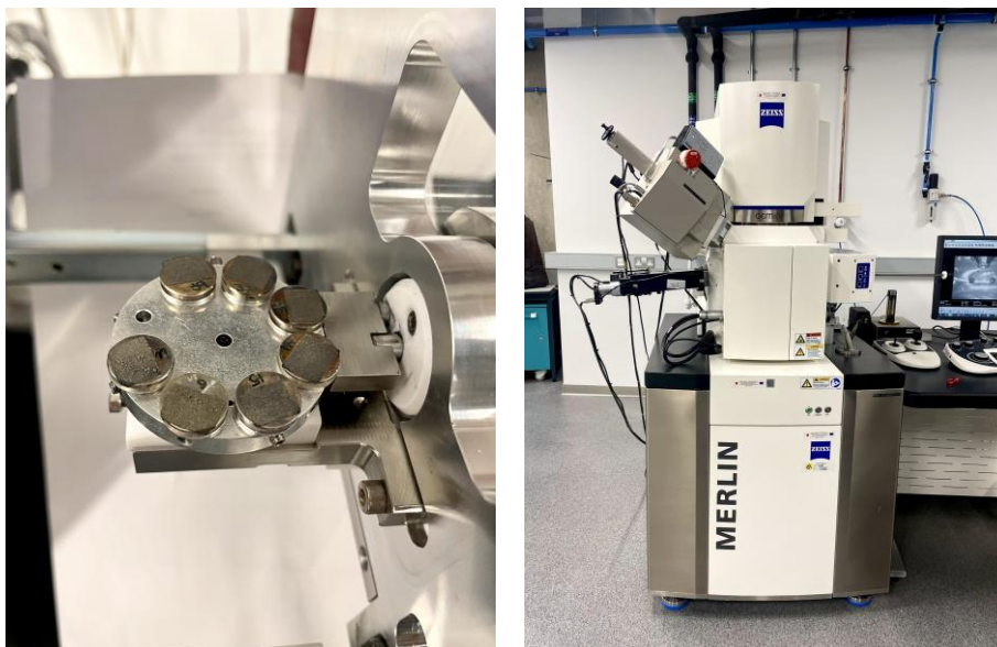
Figure 24 - Samples Prepared for SEM-EDS Testing (Left) and SEM Machine (Right)
