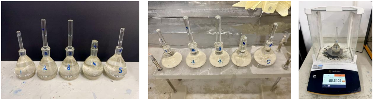
Figure 21 – Pycnometers Completely Filled with Redistilled Kerosine (left), Pycnometers Immersed in Water Bath (Middle) and Pycnometer being Weighed (Right)
