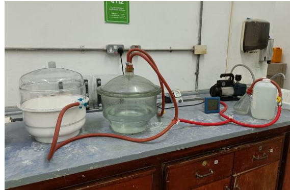
Figure 32 - Diagram of Vacuum Saturation Porosity Set Up (Left) and Vacuum Saturation Porosity Set Up (Right)
