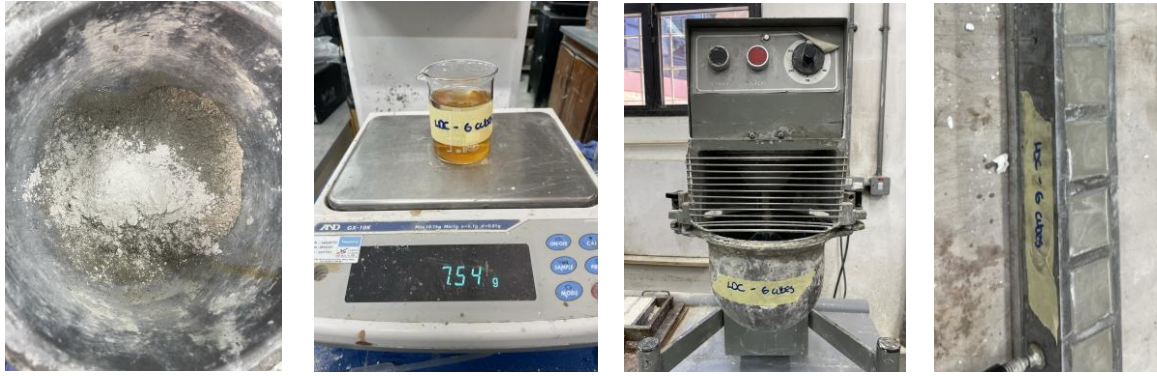
Figure 16 – Sand and Binder Mix (First), Distilled Water with Superplasticizer (Second), Mixing of Mortar (Third) and Mortar Mix placed within Mould (Fourth)
