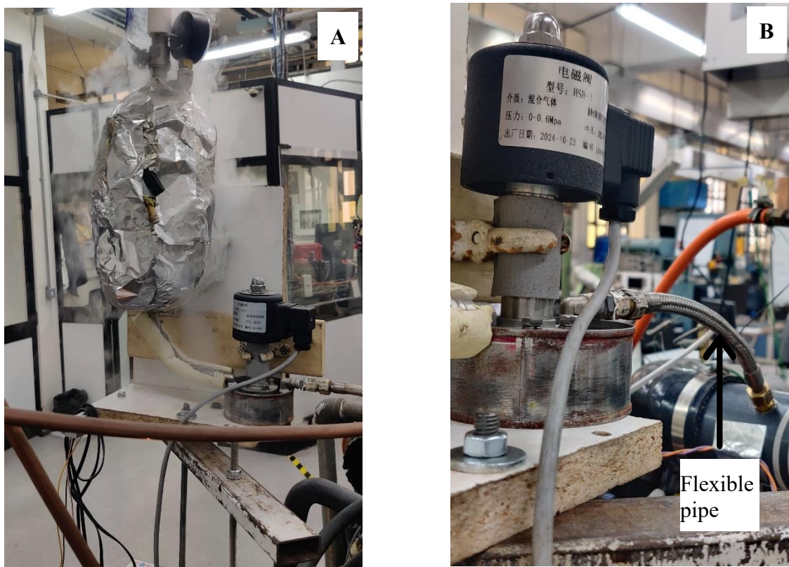
Figure 5-5: A) Installed cryogenic setup on the engine.
