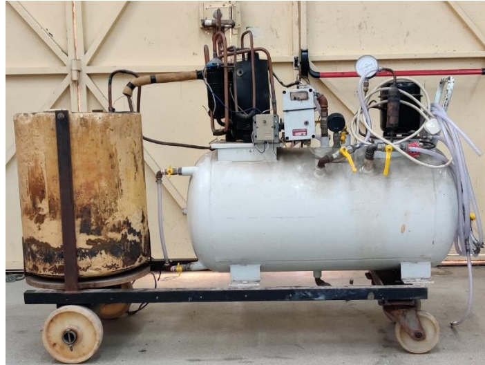
Figure 5-14: The LPG transfer unit.
