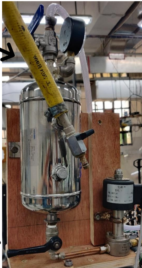
Figure 5-15: Modified cryogenic setup for liquid propane injection.
