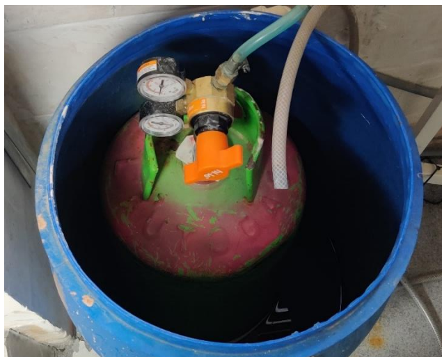
Figure 5-12: Partially submerged gas tank cylinder in water.
