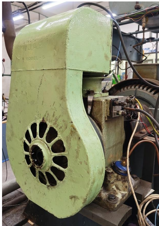
Figure 4-1: J.A.P model 6 engine used during H 2 testing.
