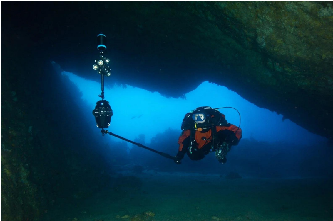
Figure 1: Insta360 Pro2 inside Mantis Sub housing with lighting rig mounted above: Image Credit: Andrew Simpson
