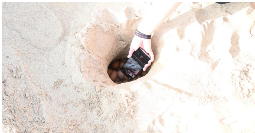
Figure 18. Scanning of the simulated sea turtle nest using a mobile application employing LiDAR technology. The device was used to capture the internal structure and wall texture of the nesting chamber.
