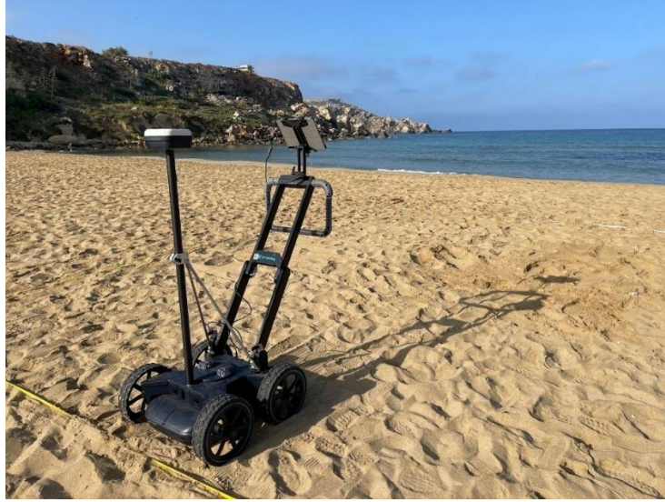
Figure 12. Ground penetrating radar (Emanuele Colica, 2025).
