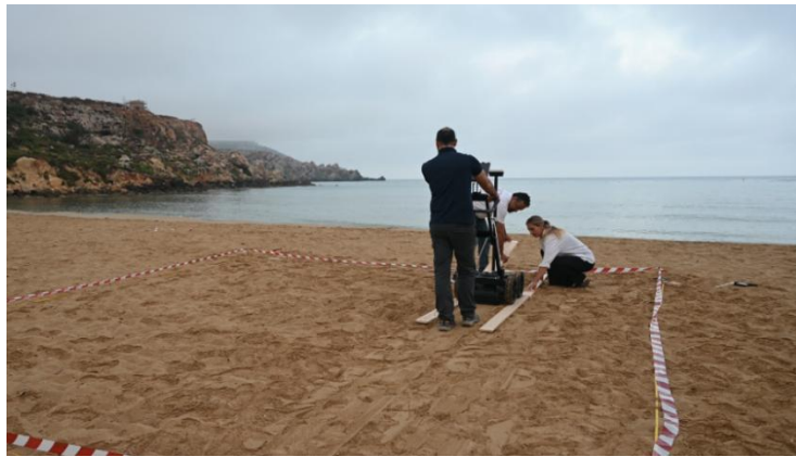
Figure 20. GPR survey conducted in the designated experimental area.
