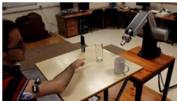
Real-time wrist position control application
