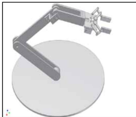
CAD drawing of the 5-DOF Control Lab manipulator
