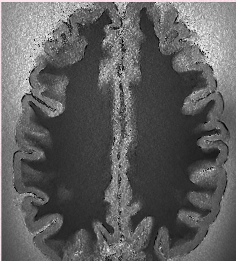
T1-map of the brain phantom, showing contrast between grey matter and white matter compositions Photo courtesy of the SARA team
