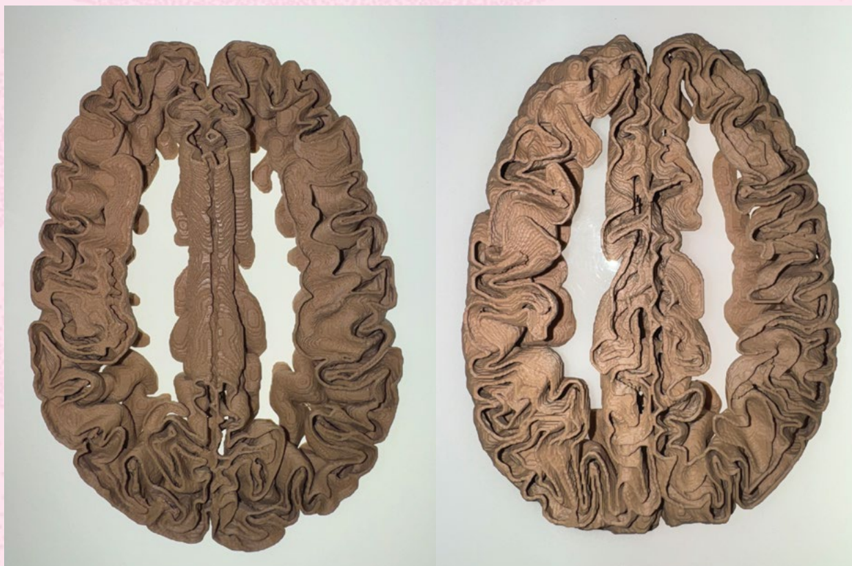
3D-printed brain slab used for phantom production – bottom view (left) and top view (right) Photo courtesy of the SARA team
