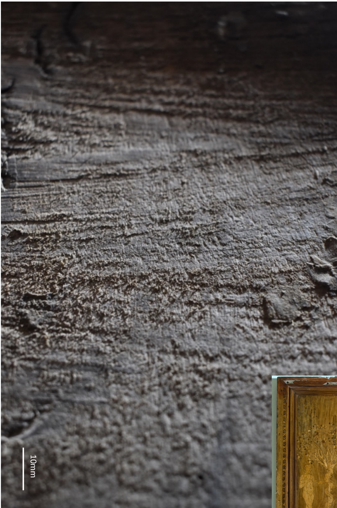
Fig. 84. Detail of the Irregular sawing marks left from original milling, on the back side of the Adam and Eve panel (inset). (James Saliba, 2024)
