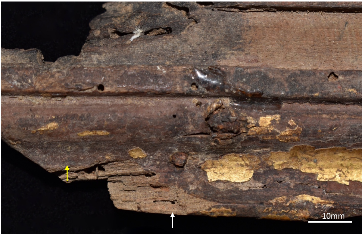
Fig. 102. Detail of an original 15th-century frame from the lower-tier frieze, revealing non-original application of grain obscuring finish. (James Saliba, 2024)
