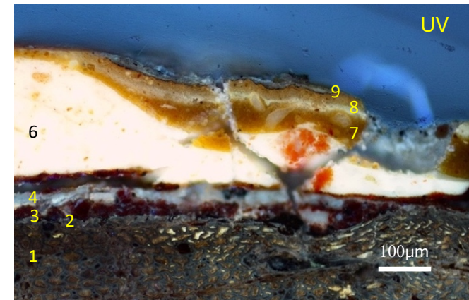
Fig.11. - Micrograph of CSM02_SC at 100x under UV light Layer 2 was visible only under UV light Layer 5 is not captured in this micrograph
