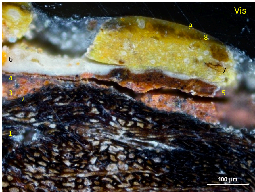
Fig.14. - Micrograph of CSM02_SC at 200x under Visible light Highlighting the presence of Layer 5
