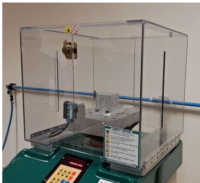
Figure 3.21: PQ1 in enclosure on the Avex SM-105 Shock Test Machine
