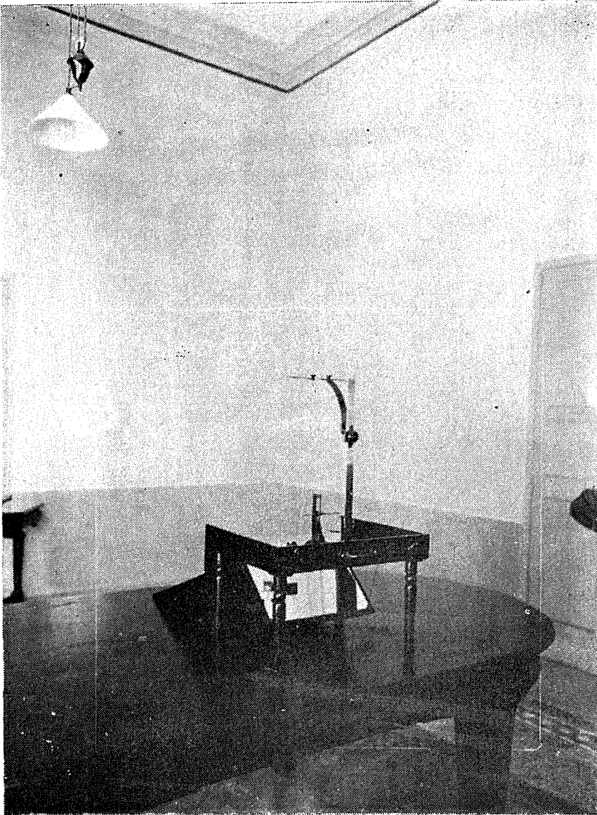
Fig. 5: The Mackenzie-Davidson Localiser for accurate determination of the position of foreign bodies employed by army medical units in Malta during World War I. (Courtesy of Mr. Richard Ellis, Valletta).
