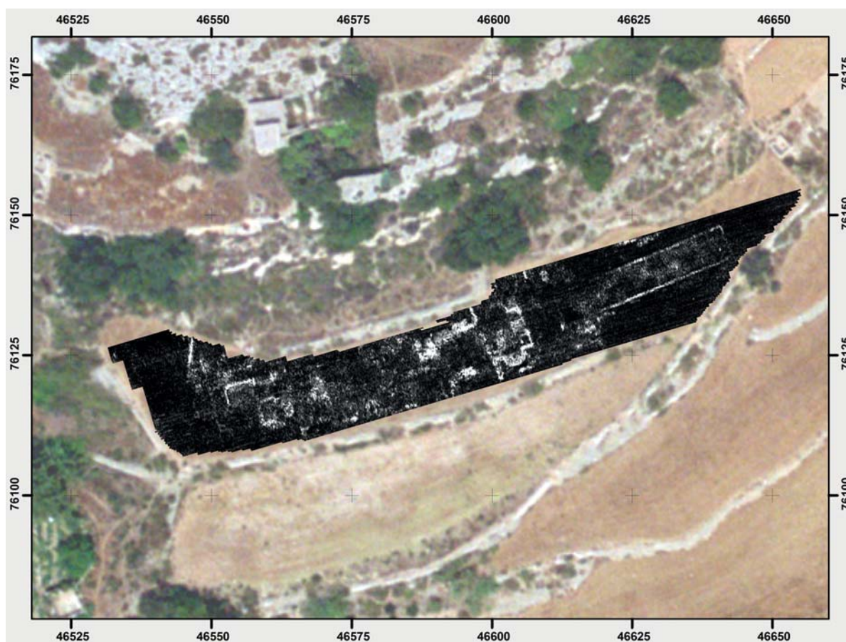
Fig. 17. Horizontal Ground Penetrating Radar (GPR) slice from tract B55 at an estimated depth of 0.80-0.85 m, projected onto an orthophotograph of the area. On the GPR slice, white areas represent strong reflections indicating the presence of buried structures; in the dark areas, radar waves were not reflected or the reflection was weak (Image: MSP, prepared by LV).
