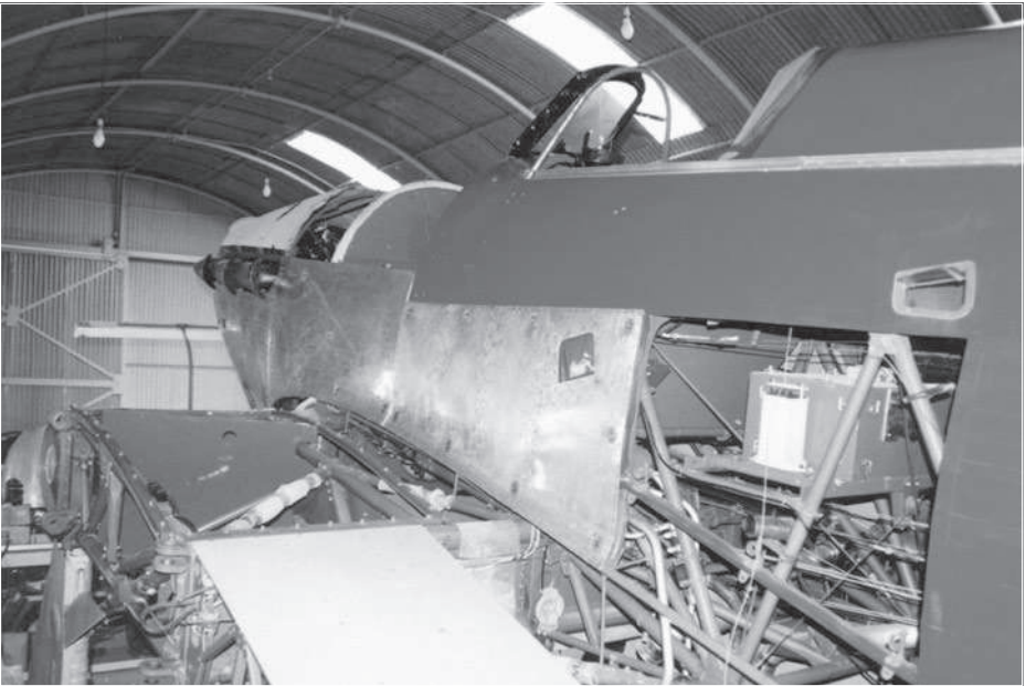
Figure 2. The painstaking restoration and rebuilding of the Hawker Hurricane Z3055 in progress, a few years after its recovery.
