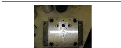
Fig. 4. Secondary Insert Holder Assembly Fitted into the Primary Mould.
