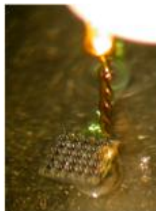
Sensor patch used to measure neural activity
