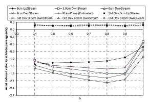
Figure 4 – Axial induced velocity distributions at blades obtained from hot-film measurements
