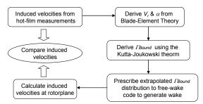
Figure 6 – Procedure for validating free-wake model using hot-film measurements
