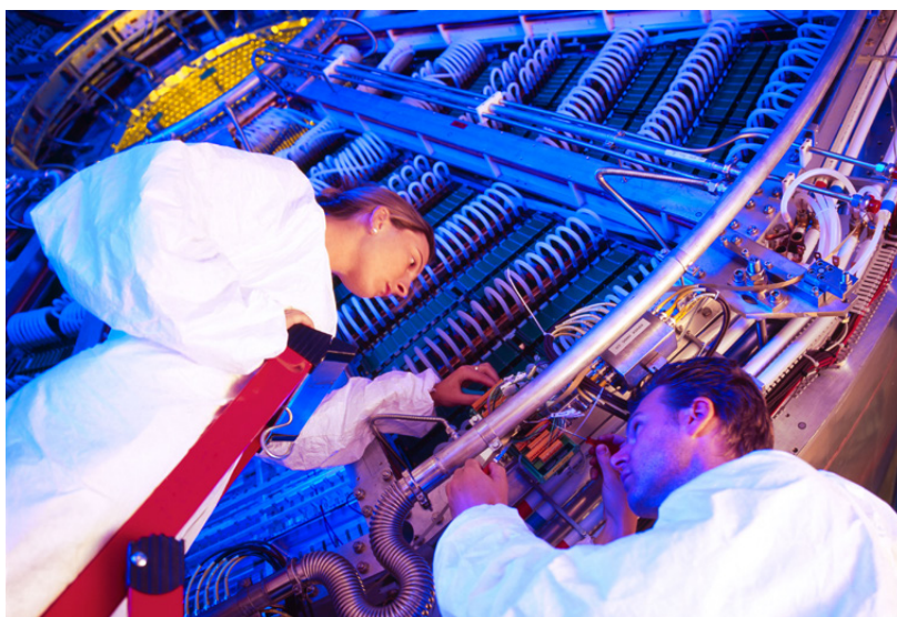
Checking the readout electronics of the ALICE Time Projection Chamber (TPC). Photo by Saba, A.
