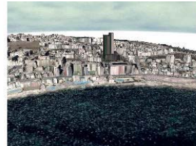
Fig. 12 Overlaying the orthoimage onto the 3D model, proposed tower development. Source: CONCHIN (2005)
