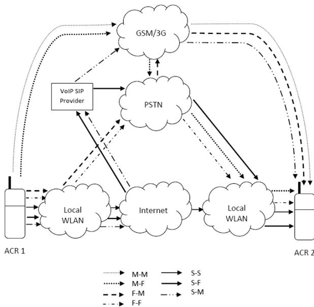
Fig. 2. The ACMR in a system that comprises cellular networks (M), PSTN switched systems, internet systems (S) and low-power radio systems that piggyback on fixed PSTN lines(F).
