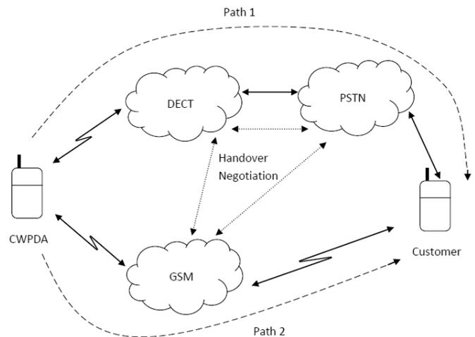
Fig. 1. A combined DECT-GSM wireless access system.
