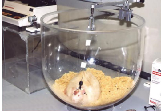
Fig. 4. Photograph of “in vivo freely moving” microdialysis setup. It is formed by a dual-channel microdialysis swivel, head block tether, and lever arm. The aCSF is delivered into the microdialysis probe by a microinjection syringe pump.
