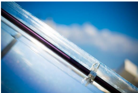
Figure 6: the coating deposited directly on a stainless steel tube
