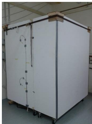
Figure 1: Hot box setup inside the laboratory at the
