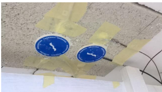
(b) Bottom part of the HCB with the 2No heat flux sensors and corresponding thermocouples installed on the web and cavity faces.
