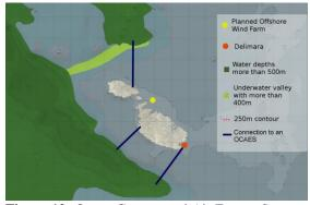
**Figure 12:** Ocean Compressed Air Energy Storage: suitable areas in relation to the Maltese islands.
