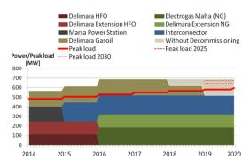
Figure 3: Scenario showing peak demand projections with changes in electricity generation and import capacity in future years (excluding renewables).
