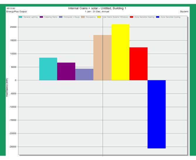
10 % reduction in cooling energy over reference scenario, however this saving in cooling energy represents only 1.16 % of the total  $CO_2$  of the Reference scenario total  $CO_2$  emissions
