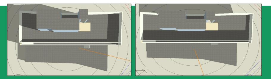
Roof shading on 21<sup>st</sup> December at 10:00 (left figure) and at 14:00 (right figure)
