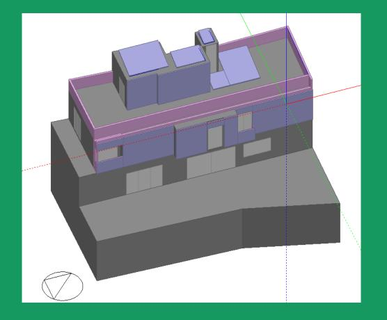
Option A – All RE panels on roof and facade are PVs with a power density of 187.5  $W_p/m^2$
