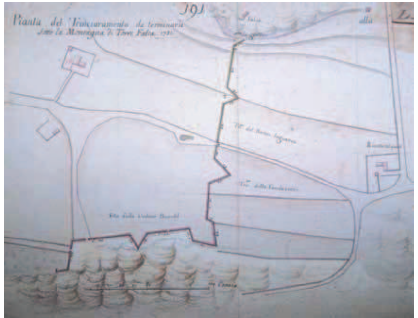
Fig. 11. Plan showing the entrenchment designed to plug the Falka Gap from the steep escarpments of Xifer il-Kief (bottom) to Dwejra heights (top). The escutcheons mounted on pillars stood on either side of the road at the point where it interrupts the entrenchment. The annotation ‘Terreno della Fondazione’ refers to Fondazione Paola. The position of Falka Tower is clearly indicated, and coincides with the position of the Roman structure. ‘Grotte’ records the presence of caves nearby, which have yielded evidence of prehistoric use. (Photo by Dr Stephen Spiteri, by kind permission of the Director, National Library of Malta).
