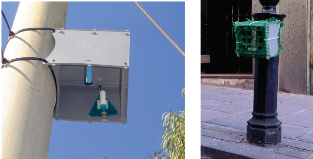
Figure 1: Left: Protective shelter used at the usual measuring height of ca. 3 meters. Right: Shelter with special protection for measurements at ca. 0.6 meters
