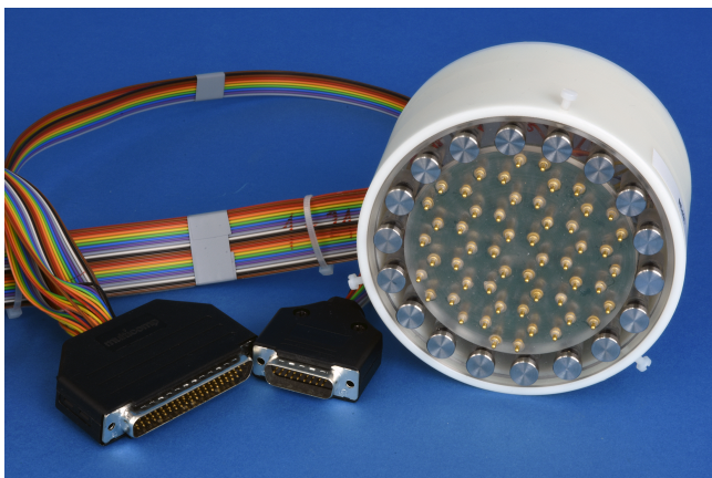
Figure 2: Sensing head of the EIM device developed at the University of Mainz in collaboration with the University of Malta and Oxford Brookes University.
