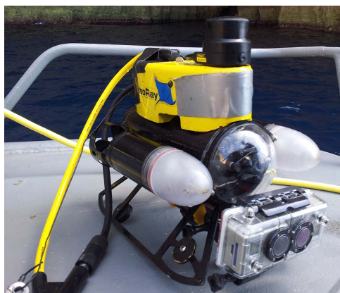
Figure 2: The VideoRay Pro III GTO is an underwater micro-ROV (36.8 cm x 28.9 cm x 21.6 cm), with a depth sensor, a compass, and a front and rear video camera. A removable Tritech Micron scanning sonar was mounted to the top and two vertically aligned GoPro Hero2 cameras were mounted to the front in a waterproof stereo casing.
