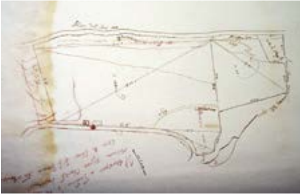
Fig. 10: NLM, Treas. B. 291, f. 86. Plan of the Tal-Callus giardino . This is a more detailed version of the plan of the Tal-Callus estate (RA39) on which that included in NLM, Treas. B. 290, f. 77 was produced. Clearly indicated is the location of two fontane first mentioned in NLM. Treas. B. 289, f. 84. The transverse triangulations included in the plan suggest that this was probably drawn on site
