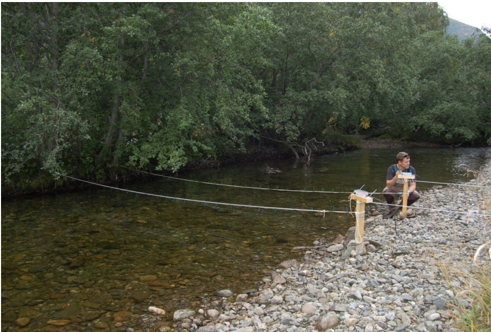
Figure 2.3.5.17: PIT detector station in a Norwegian stream. The wires seen crossing the river form part of the loop antennae.
