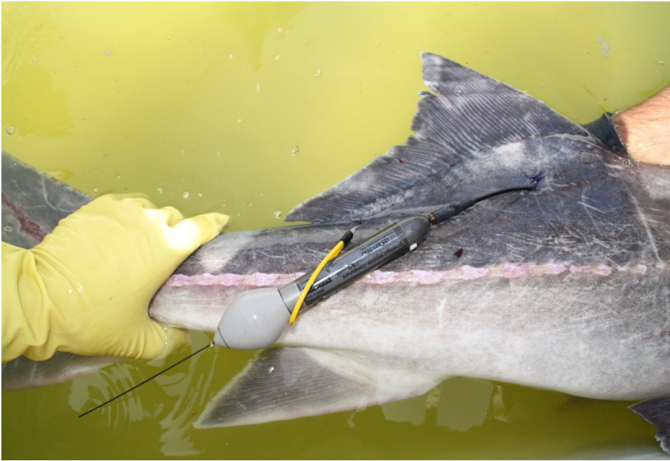
Figure 2.3.5.19: PSAT installed in the dorsal region of a sturgeon.
