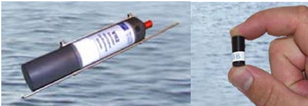
Figure 2.3.5.14: Automated omnidirectional receiver (left); miniaturized ultrasonic transmitter ( pinger ) (right) (from www.vemco.com ).
