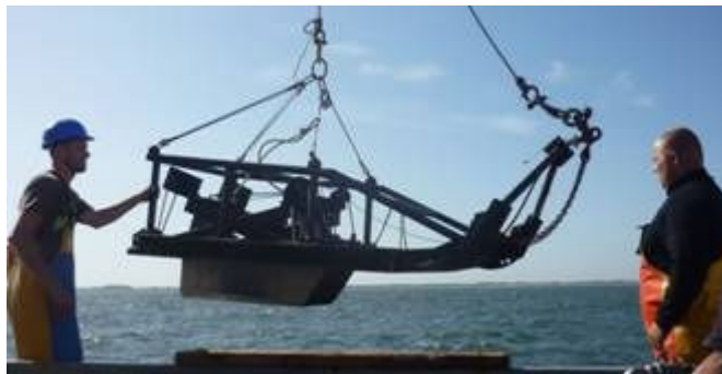
Figure 2.3.6.13: The semi-grab, a device designed to sample deep burying bivalve species.
