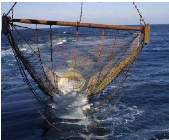
Figure 2.3.5.6: 8m beam trawl at the start of the haul (left); scheme of the beam trawl net used in the Dutch beam trawl survey (right).
