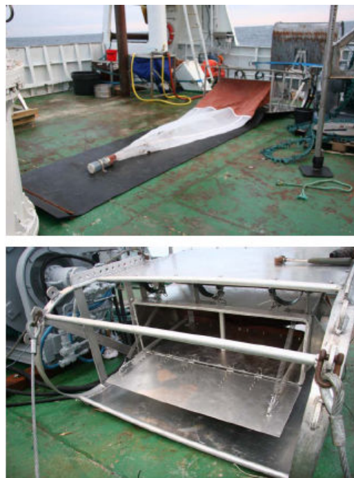
Figure 2.3.6.2: Details of a hyperbenthos sledge (see Buhl-Jensen, 1986; Brattegard and Fosså, 1991; Miskov-Nodland et al., 1999) showing (top) the fine mesh collecting net extending back from the Sledge-mounted rectangular sampling box, and (bottom) the front end of the sampler with Spring-loaded opening/closing mechanism.
