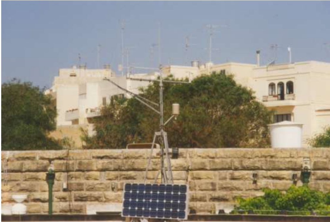
Figure 3: A weather station on the roof of the Institute.
