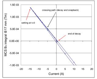
Figure 2: Spool pieces sextupoles integrated strength as a function of current, simulating the compensation of decay and snapback of b3 in the main dipoles of sector 7-8.
