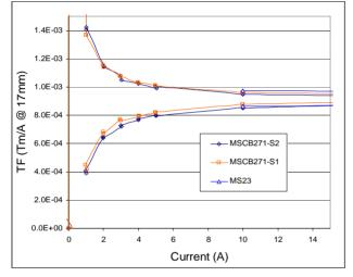
Figure 1: Lattice Sextupoles transfer functions as a function of current.
