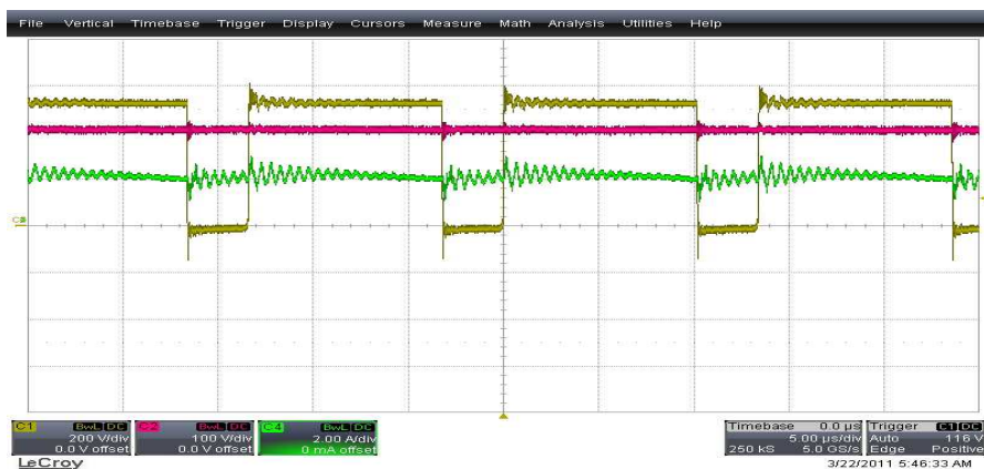
Figure 10: Dc-Dc converter operating at full load at an input voltage of 400V V_{DS} (Yellow) V_O (Red) I_{IN} (Green)
