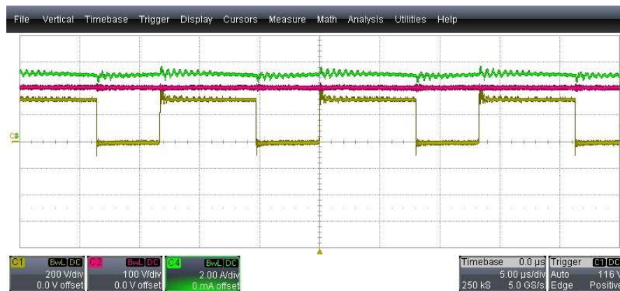
Figure 9: Dc-Dc converter operating at full load with an input voltage of 200V V_{DS} (Yellow) V_O (Red) I_{IN} (Green)
