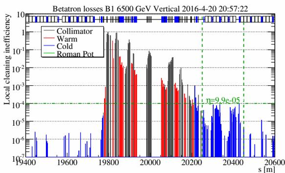
Figure 3: Distribution of beam losses in the LHC ring zoomed in IR7 for Beam 1 vertical betatronic losses. The loss signal for each BLM is normalized to the maximum loss.
