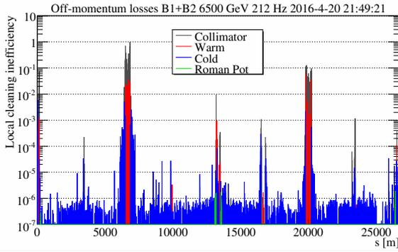
Figure 2: Distribution of beam losses in the LHC ring for Beam 1 and Beam 2 off-momentum losses. The loss signal for each BLM is normalized to the maximum loss.
