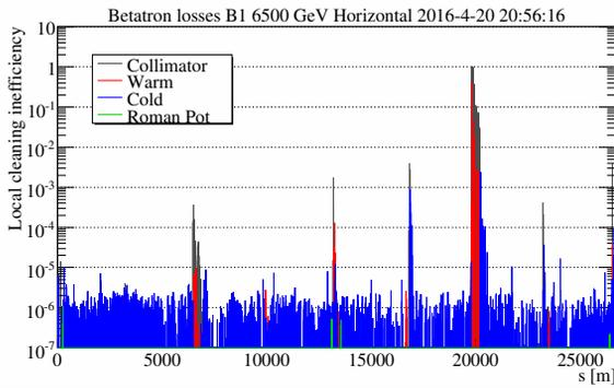
Figure 1: Distribution of beam losses in the LHC ring for Beam 1 horizontal betatronic losses. The loss signal for each BLM is normalized to the maximum loss.
