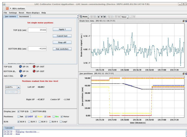
Figure 2: RP movement sequence during the interlock tests 2011: black = motor step counter position, blue = LVDT position, red = outer and inner dump limits, yellow = outer and inner warning limits. At 19:26:40 the inner limits are changed such that the RP position becomes illegal. Consequently the pot is automatically retracted. The LVDT correctly indicates the new position ( \sim 39.7 \text{ mm} ). The step counter, however, stays at 37 mm because in the emergency extraction with the springs the motor coupling is lost. A reset at the mechanical reference point (OUT stopper) is needed.
