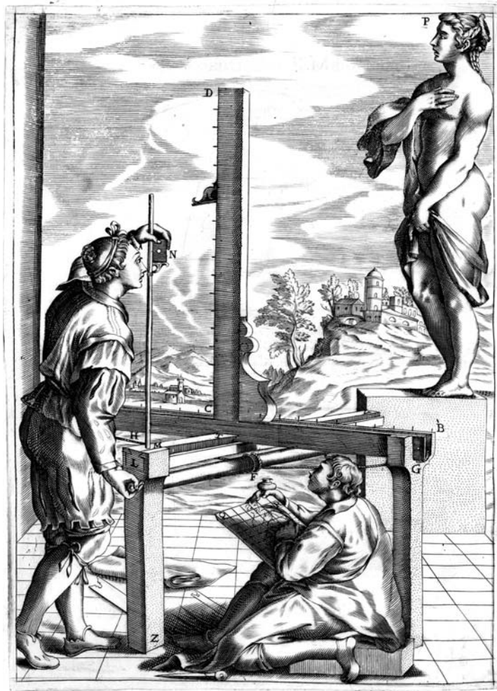
Figure 33: Jacopo Barozzi's Perspective Machine. (Kemp, 1990, p. 174)
