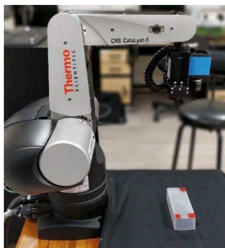
Figure 3.3: The eye-in-hand visual servoing system
