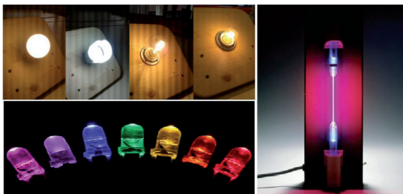
Figure 1. Different kinds of lamps are used in the path: incandescent, halogen, fluorescent, white and coloured LEDs, gas discharge.
